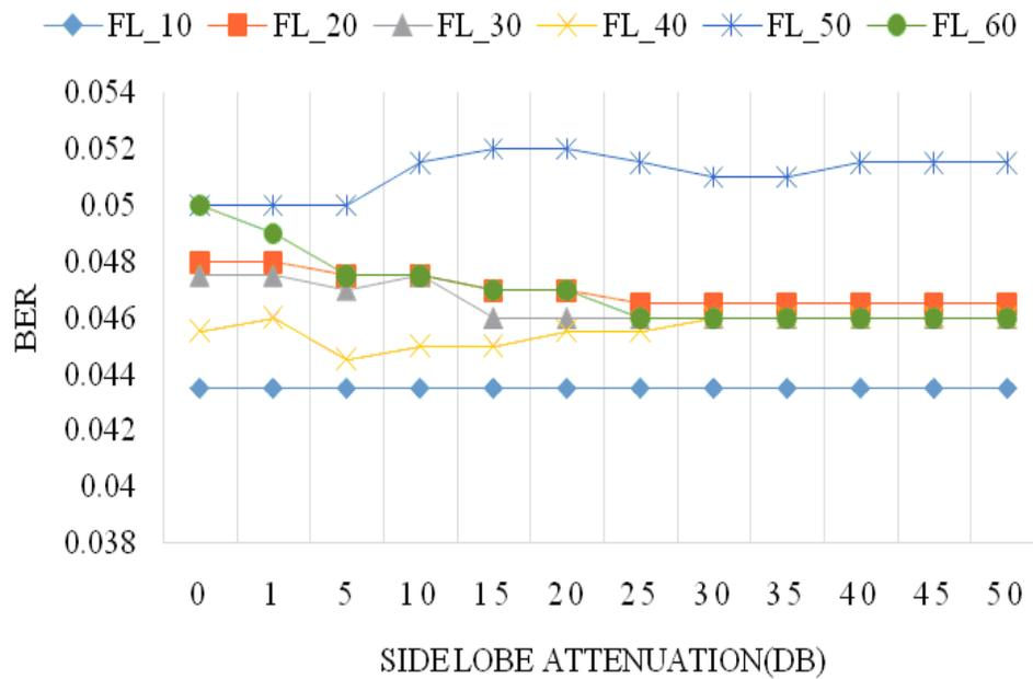
**Figure 3:** BER of given filter length for various side-lobe attenuation
