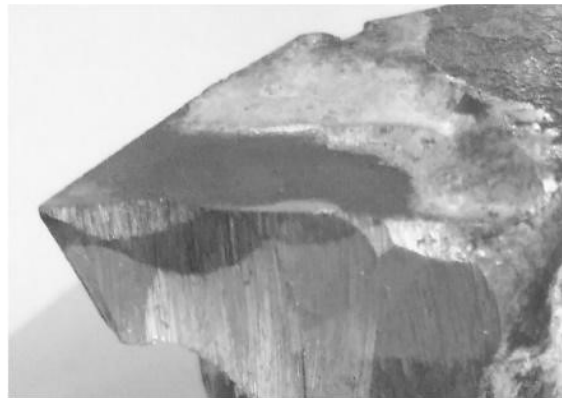
Fig. 11. Gray level image of the tool after machining
