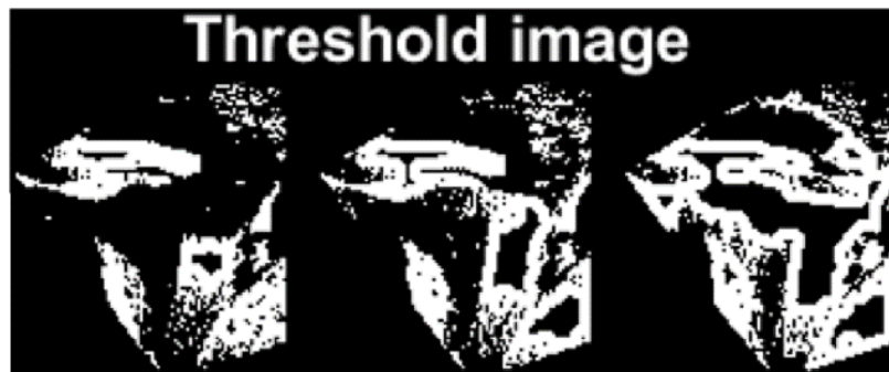
Fig. 14. Edge detection of the wear in the image of the tool after machining
