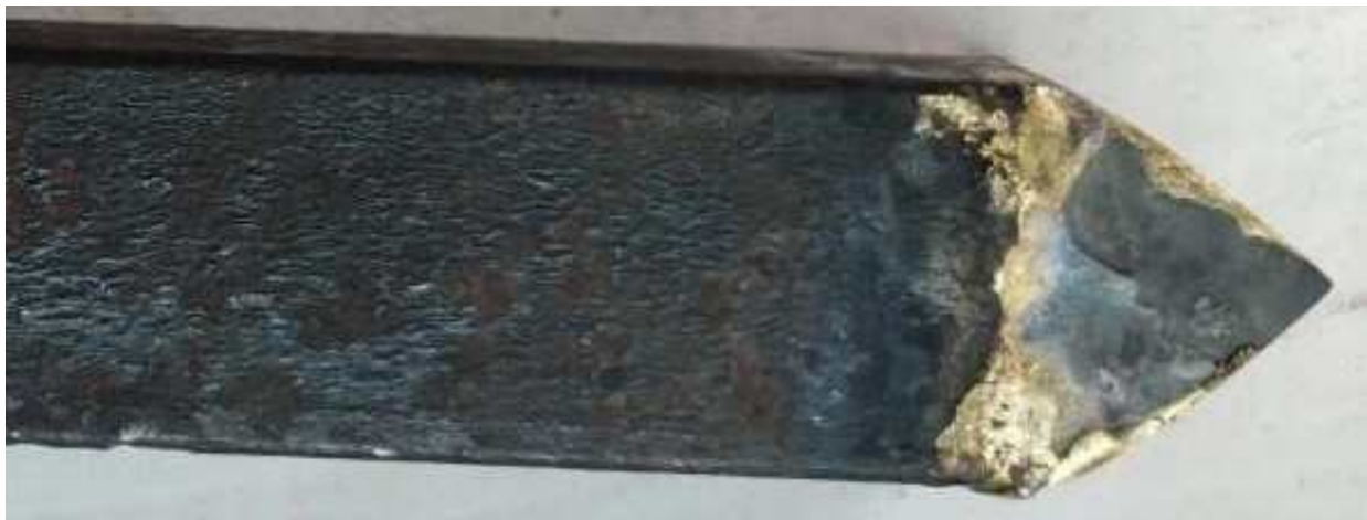
Fig. 3. Carbide insert welded with the iron shank
